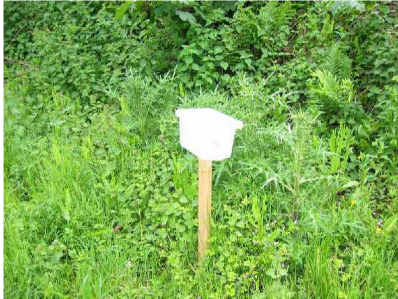
Image 5.2 A plastic box used for housing an automated bat detector along a hedgerow
