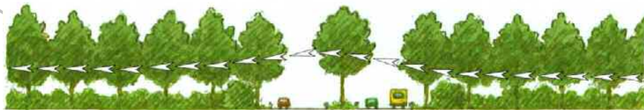
Image 8.10 'Double hop overs' should be considered for wide roads such as dual carriageways; by planting in the central reservation the space between tree canopies is reduced.
