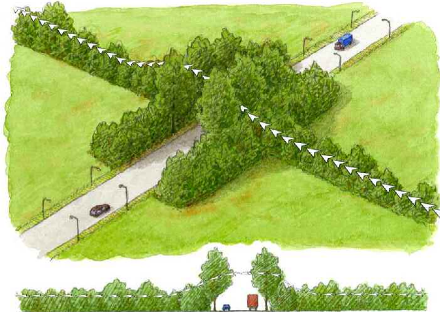
Image 8.9 'Hop over' – bats can be encouraged to fly high over road and traffic by enhanced planting and use of lighting columns; allow tree canopies to touch if possible.
